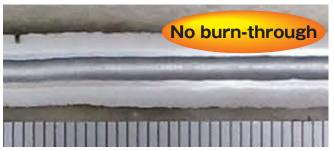
Weld conditions: ·Base metal: A5052 ·Joint: Butt ·Weld current: 50 A ·Weld speed: 150 cm/min ·Plate thickness: 0.6 mm
