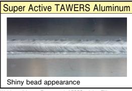
Weld conditions: ·Base metal: A5052 ·Joint: Fillet ·Weld current: 155 A ·Weld speed: 60 cm/min ·Plate thickness: 3.0 mm
